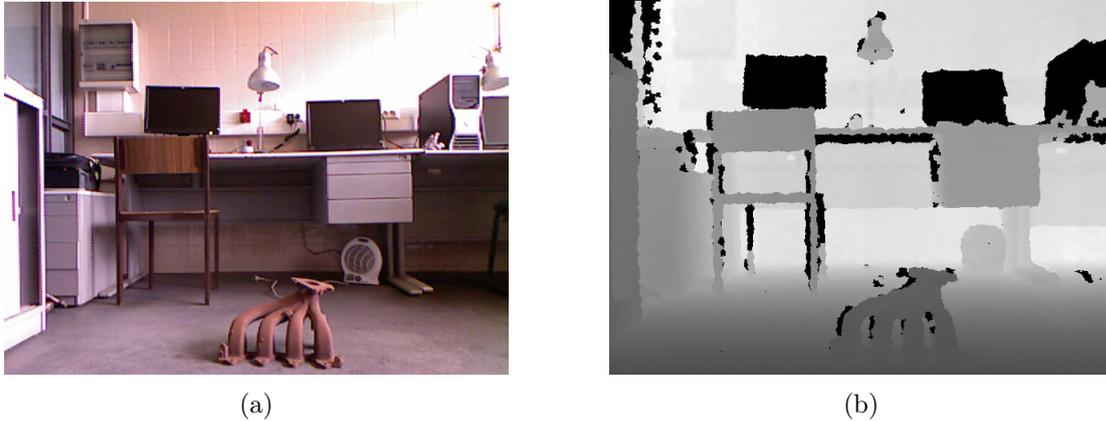
Figure 5.1: RGB image (a) and depth data (b) acquired by Kinect
