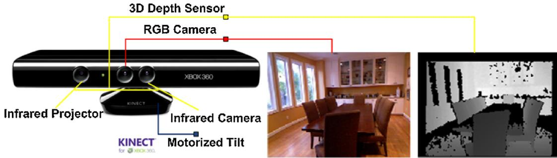
Figure 2.3: Hardware configuration of Microsoft Kinect, and two image samples captured [10].
